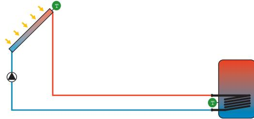
Internal heat exchanger, intelligent pump control
